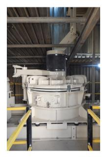
to produce such fine material. But a mill is a very costly machine and producing aggregates at the same time would be only possible by using an additional crusher. The solution from Quarry Mining was the use of a vertical impact crusher (VSI) and 2-deck screen in combination with a cascade sifter system connected to the dedust plant. Like this the third critical issue could be solved.
