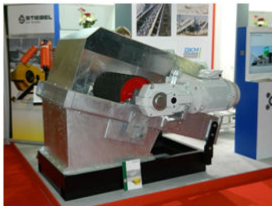
Conveyor system with Stiebel gearmotor
