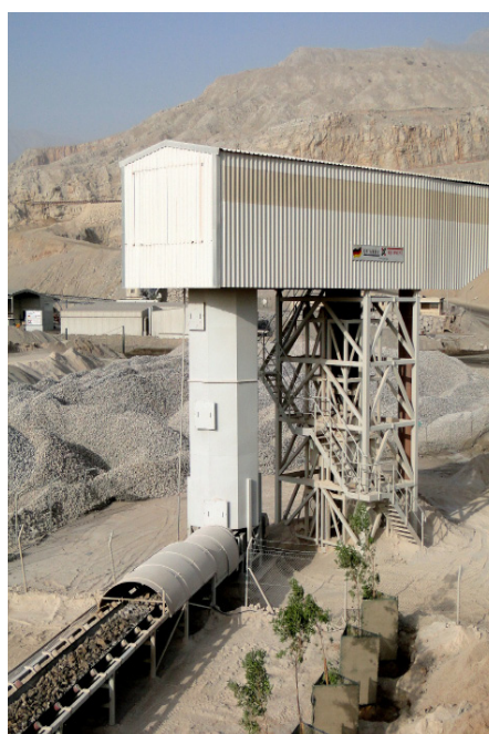
Stone ladder dropping the material 9m step by step onto a conveyor
