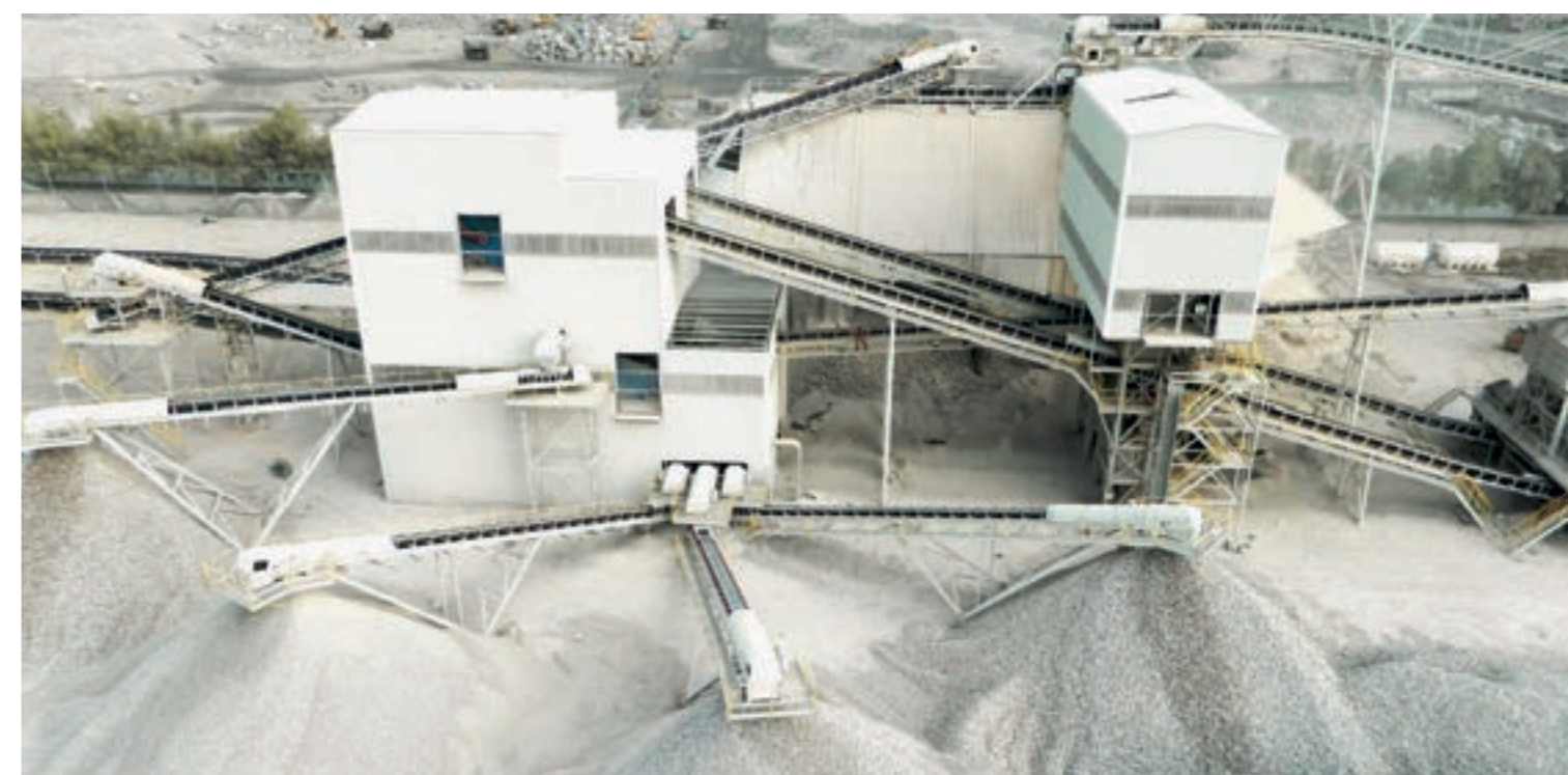
Stationary primary and secondary crushing plants of different capacities (from 350 tph feed up to 3500 tph feed)
